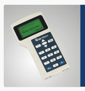
Reliable and convenient handheld service unit is necessary for uploading programs and data transfer to electronic door locks and safes.
